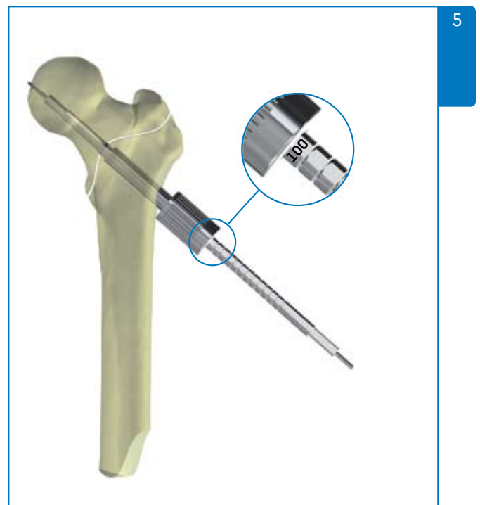
Set the three step milling cutter (S106) on the measured length and perform milling
